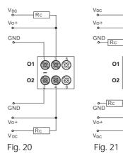
**Open collector outputs:** The load resistance (Rc) must be calculated so that the closed contact current is lower than 100mA; the VDC voltage must be lower than or equal to 30V. VDC: power supply voltage (external). Vo+: positive output contact (open collector transistor). GND: ground output contact (open collector transistor).
