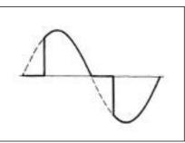
Figure BSine wave, indentedFundamental content10...100%Harmonic content0...90%Frequency spectrum:3rd to 16th harmonicAdditional error: <1% FS</td>
