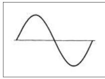
Figure ASine wave, undistortedFundamental contentHarmonic content0% $A_{rms} =$ 1.1107 |  $\overline{A}$  |
