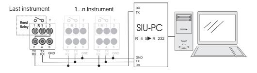
2-wire connection of RS485 serial port + one relay (R). The terminalization must be carried out only on the last instrument of the network
