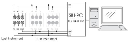
4-wire connection of RS485 serial port, the terminalization must be carried out only on the last instrument of the network
