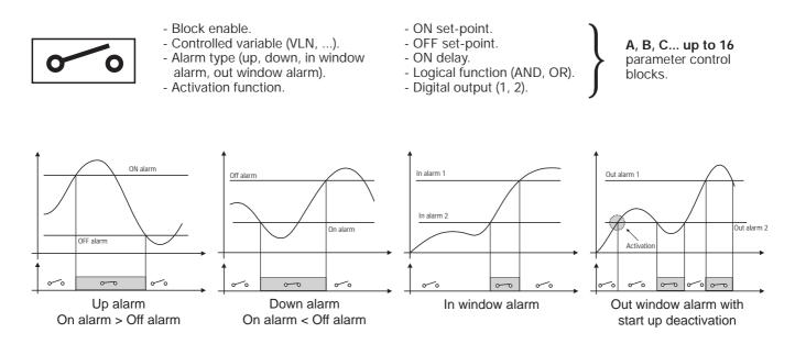
Note: any alarm working mode can be linked to the "start up deactivation" function which disables only the first alarm after power on of the transducer.
